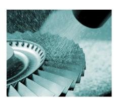
Manufacturers in the aerospace, automotive, infrastructure and other critical industries rely heavily on automated shot peening to boost the performance and service life of their high-strength metallic products and parts. This is because important metal parts that are subject to frequent forms of stress may fail prematurely through a fracture that begins at the surface, leading to potentially disastrous results.
