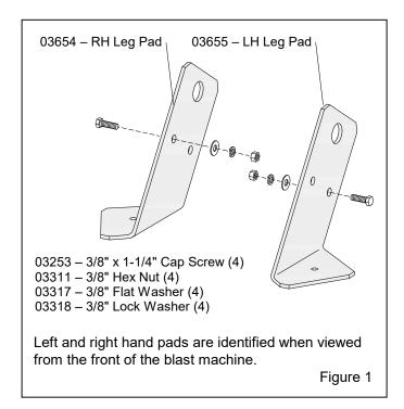
1.3 These instructions explain how to remove the wheels and attach leg pads one side at a time, which is the easiest method if lift equipment is not available. If appropriate rigging or blocks are available, lift both sides and block the axle pipe only enough to spin both wheels freely.
