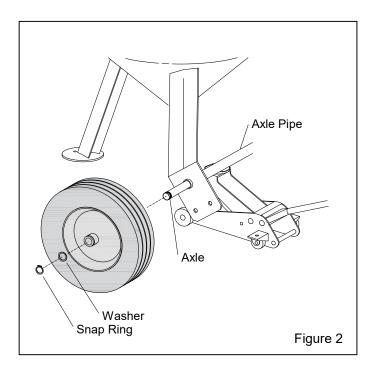
**2.3** Remove the snap ring and washer, and then slide the wheel off the axle.
