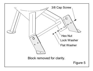
**4.4** Remove the block. Holes in the pads and front leg are to anchor the blast machine to the floor for stability.
