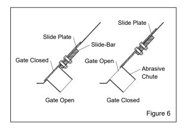
**3.3 To close the slide-gate,** loosen the nuts on the slide-bar and slide the gate down, as shown in Figure 6; this moves the slide plate over the abrasive chute and stops abrasive flow in the blast machine. Snug the lock nuts to secure the gate in the closed position.
