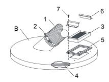
Cover for blast machine without a flange.
