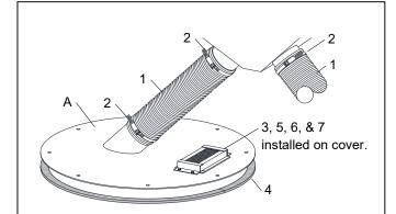
Cover for blast machine with a flange.
