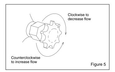
**4.1.3** The valve is closed when the knob is turned fully clockwise. Begin with the knob set 1-1/2 turns from fully closed. To increase abrasive flow, the machine tender turns the knob no more than 1/4 turn counterclockwise while the operator is blasting. Allow 10 to 15 seconds for the flow to stabilize before readjusting. Continue making adjustments as described until the correct flow is attained. The valve is fully open when the knob is turned fully counterclockwise.
