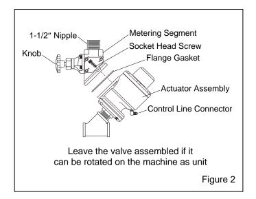
**2.2.4** Remove the four socket head screws holding the metering assembly to the actuator, and remove the actuator assembly.
