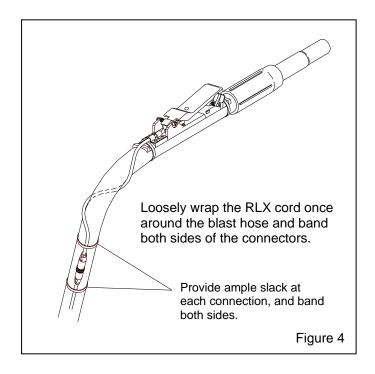
**2.3.9** Band the cord to the blast hose every 4 to 6 feet. When attaching control cord extensions wrap the cord around the blast hose and band the cord on both sides of each electrical connection.
