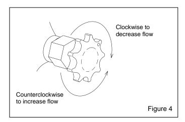
**4.1.4** Optimum abrasive flow depends on the type and size of abrasive and blasting pressure, and can best be determined by experience. Use as little abrasive as possible while maintaining the maximum cleaning rate. The air/abrasive mixture should be mainly air. As a rule, the stream of abrasive coming out of the nozzle should barely discolor the air when seen against a contrasting background.
