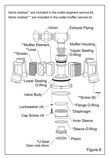
**6.4.9** Verify that the inner sleeve o-ring is in the lower groove, not in the upper groove which has the vent hole.
