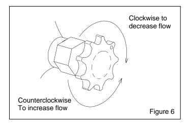
**4.1.4** The valve is closed when the knob is fully clockwise. Begin with the knob set 1-1/2 turns from fully closed. While the operator is blasting, the machine tender turns the knob no more than 1/4 turn counterclockwise to increase abrasive flow. Allow 10 to 15 seconds for the flow to stabilize before readjusting. Continue making adjustments as described until the correct flow is attained.
