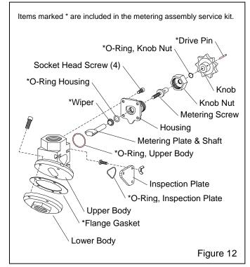
**6.7.2** If the valve requires immediate service, and the machine cannot be emptied of abrasive, turn the adjusting knob fully clockwise to shut-off abrasive flow. If the valve is worn so that abrasive does not shut-off, remove the inspection plate, and insert a rag or similar object into the opening to block the flow of abrasive.
