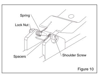
**6.6.3.2** Install a new handle lever and spring, and reassemble in reverse order.
