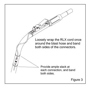
**2.2.5** Band the cord to the blast hose every 4 to 6 feet. When attaching control cord extensions, provide slack at each connection and band the cord on both sides of each electrical connection.
