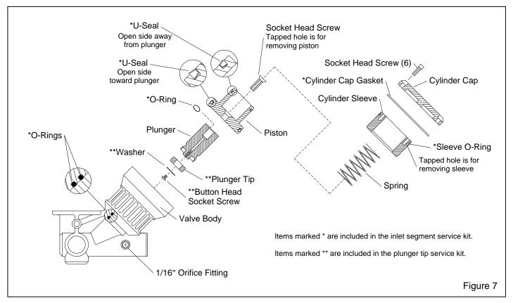
**6.3.7** If the plunger and piston were separated as noted in paragraph 6.3.4, apply removable thread sealant to the socket head screw, and reassemble the parts using a new o-ring supplied with the service kit.
