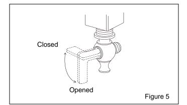
**3.2.12**Check to make sure that the handle lever will not engage the switch unless the safety lever lock is pulled down.
