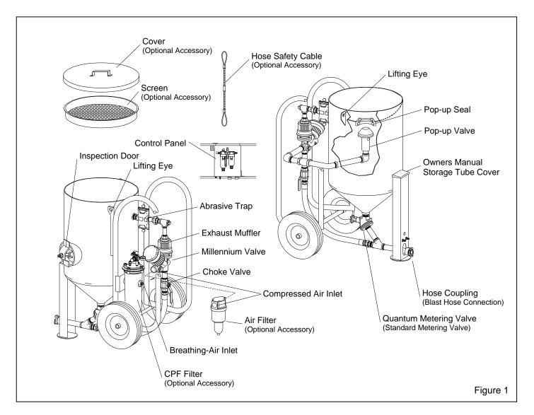
**1.3.3.5** The blast machine is equipped with remote controls that allow the operator to pressurize the machine to start blasting, and depressurize it to stop blasting, at the nozzle.
