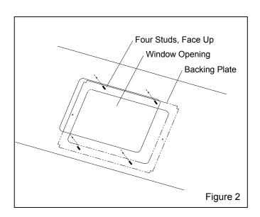
**4.2** Temporarily bolt or clamp the backing plate into position to prevent movement.
