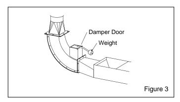
**10.1.2** Once adjusted, the damper will open to clear the M-Section® transition should it become plugged.
