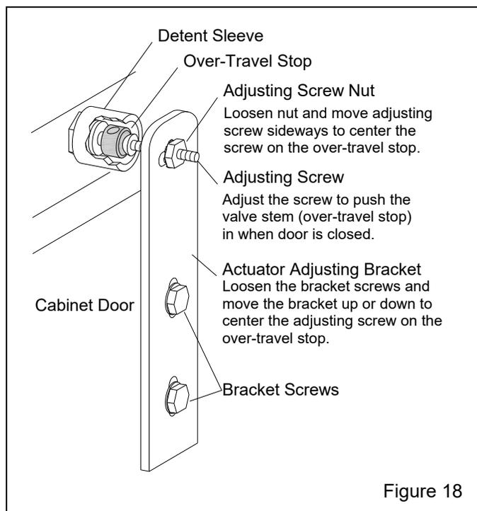
**5.7.3** Loosen the actuator bracket screws and adjusting screw nut. Move the actuator bracket up or down, and the adjusting screw sideways, to center the adjusting screw on the over-travel stop. Tighten the bracket screws.
