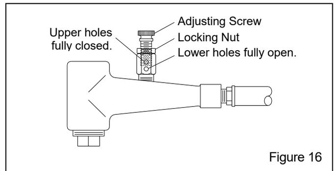
**5.3.4** If media flow is too light, decrease air in the mixture by turning the metering screw in (clockwise when viewed from the top), covering more of the holes so less air enters the media hose. Tighten the locking nut finger-tight to maintain the setting.
