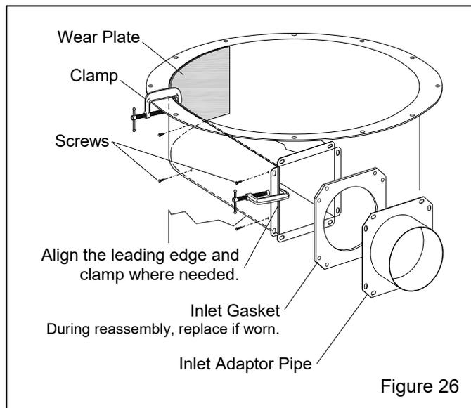
**7.8.2.6** New self-drilling sheet-metal screws are provided with the wear plate; match drill through each old screw hole into the wear plate to secure. Rearrange the clamp(s) as needed to press the wear plate against
