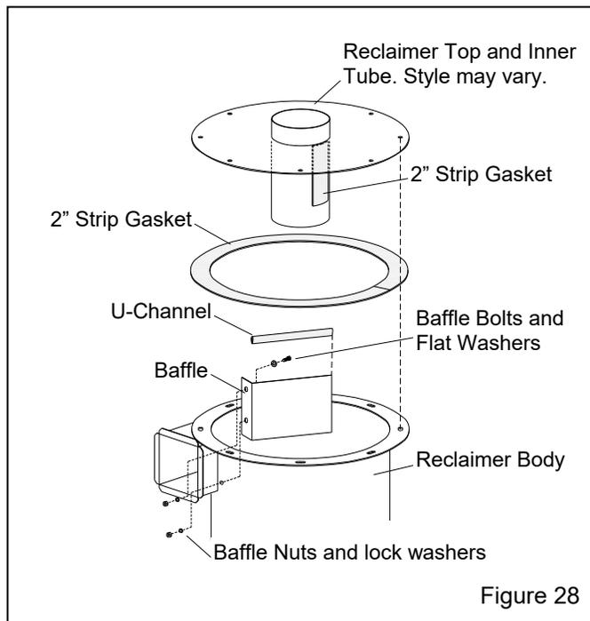
**7.10.5** If removing (not replacing) the baffle, remove the strip gasket from the inner tube, install the baffle bolts and reclaimers top. If replacing the baffle, skip to Paragraph 7.10.6.
