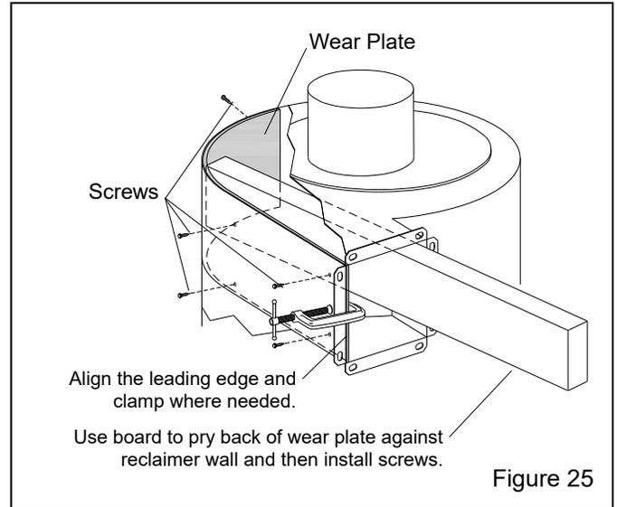
**7.8.1.9** To avoid rapid wear, apply RTV caulk to fill gaps at the seams on the top and bottom of the wear plate
