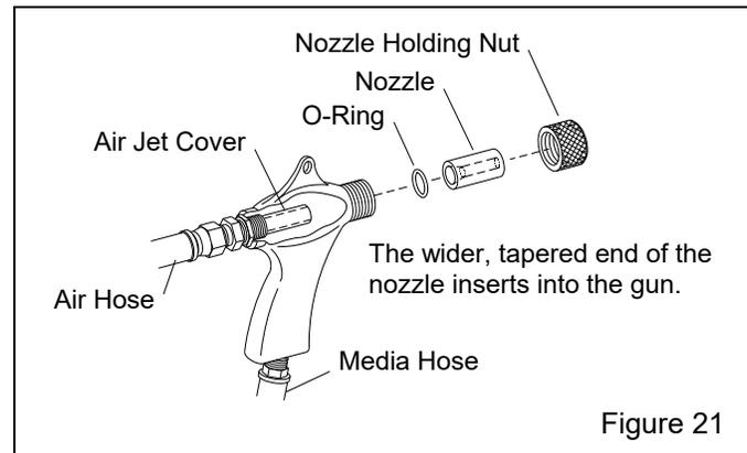
**7.2.1** Replace the nozzle when its orifice diameter has worn 1/16" larger than its original size or when suction diminishes noticeably. To change the nozzle, unscrew the holding nut from the gun end and pull the nozzle from the gun. Inspect the nozzle O-ring and replace if worn or damaged. Inspect the air jet cover; replacing it before it wears through will prolong the life of the jet. Insert a new O-ring and nozzle, placing the tapered end toward the jet. Screw the holding nut onto the gun.
