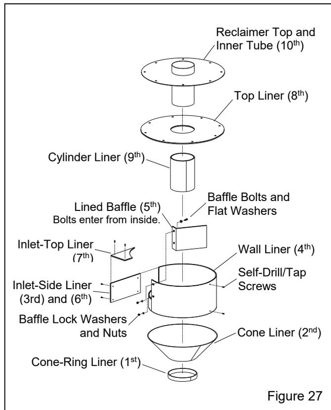
**7.9.23** (9th) Place the cylinder liner over the inner tube. Make sure the liner is tight against the top liner and use worm clamps to temporarily clamp the liner to the tube. Tack weld the bottom of the cylinder liner to the inner tube in three or four places. Remove the clamps when the cylinder liner is secured.
