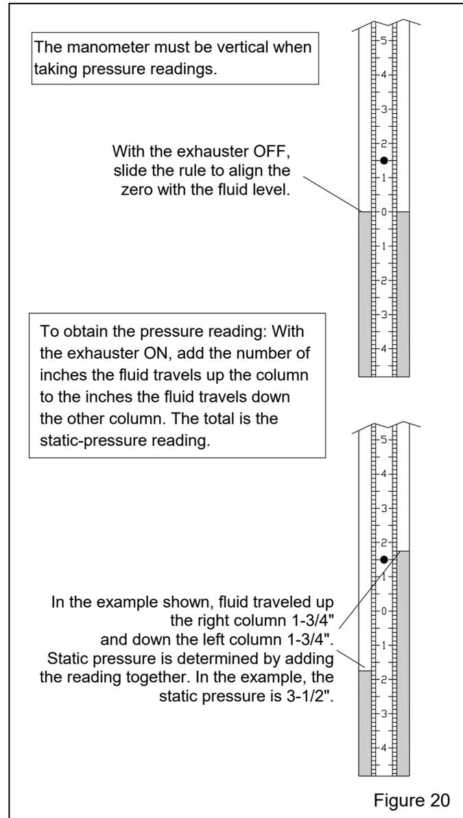
**5.8.9** To find the static pressure, add the number of inches the fluid travels up one column to the inches the fluid travels down the other column. Refer to the example in Figure 20.
