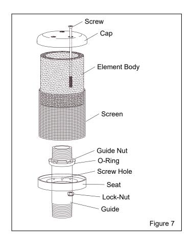
**5.10.8** Firmly tighten the lock-nuts.
