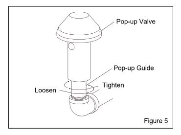
**5.7.4** While the pop-up valve is out, check alignment as follows: Screw a 1-1/4" nipple, that is at least 12"
