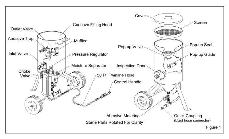
**1.3.2.3** This blast machine is rated for a maximum of 125 psi (pounds per square inch); do not exceed the rated pressure.
