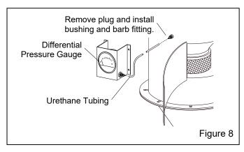
**3.4.4** Remove the 1/4" pipe plug from the reclaimer body and install 1/4" x 1/8" bushing and barb fitting, as shown in Figure 8.
