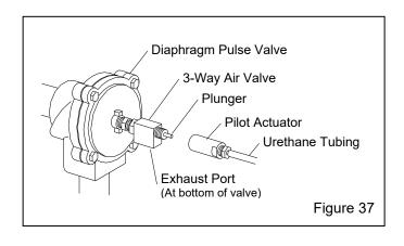
NOTE: The 3-way valve at the foot pedal and the 3-way on the diaphragm pulse valve are identical. If there is doubt as to whether either 3-way valve is functional, the valves may be tested by swapping one with the other.
