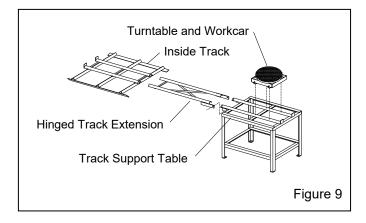
**3.5.2** Place the inside track in the cabinet over the existing grate, as shown in Figure 10.
