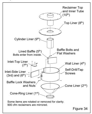
**7.13.21** (7th) Align the front edge of the inlet-top liner to the front of the inlet housing and use self-drilling screws to secure. NOTE: To field install new, first-time inlet-top
