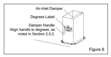
**2.5.2** Loosen the lock nuts and align the damper handle to the initial setting of 30 degrees. When correctly positioned, tighten the lock nuts to maintain the setting. Refer to Section 5.6 for adjustment procedure.
