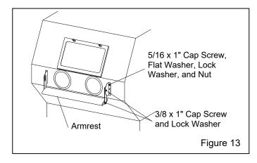
**3.7.5** Loosen the fasteners on the slotted bracket and raise or lower the armrest to a comfortable position.
