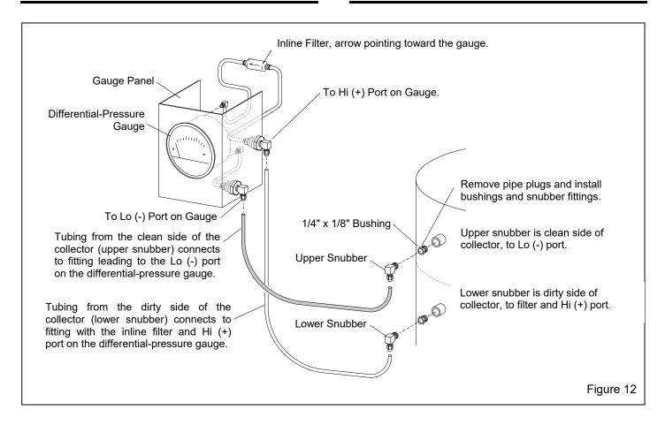
the panel. NOTE: Make sure the panel is close enough to the dust collector for 10 feet of tubing to reach.
