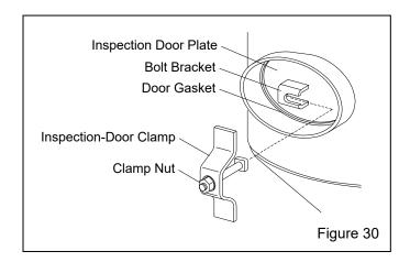
2. Push the inspection-door plate into the blast machine and rotate it so it can be removed through the inspection
