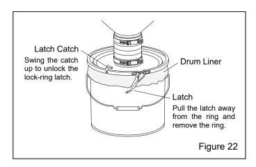
**3.** Tie off or otherwise seal the top of the liner and remove it from the container. Dispose of the sealed liner into a suitable disposal receptacle.
