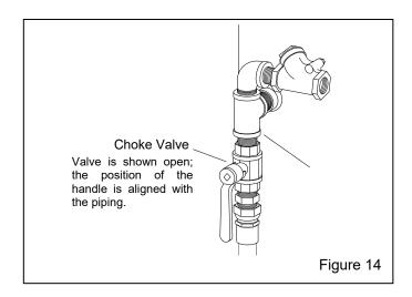
**4.6.2** Closing the choke valve while blasting lowers pressure in the pusher line from the pressure in the vessel. Closing the valve forces media through the metering valve to clear minor blockage, such as damp media, or it is used to rapidly empty the machine to change media.
