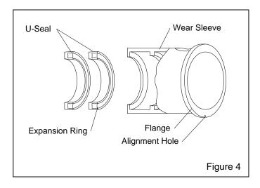
**4.4.7** Place the wear sleeve in the body. Align the hole in the sleeves flange with the pin in the body. Make sure the opening in the wear sleeve lines up with the opening in the body.
