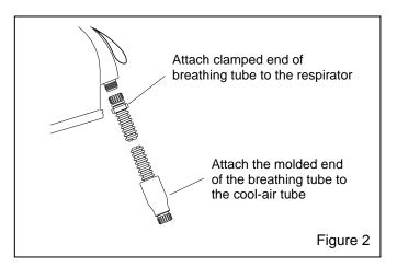
**3.1.2** Attach the clamped-on end to the threaded air inlet fitting at the back of the helmet as shown in Figure 2. Do not over-tighten; hand-tight is sufficient.
