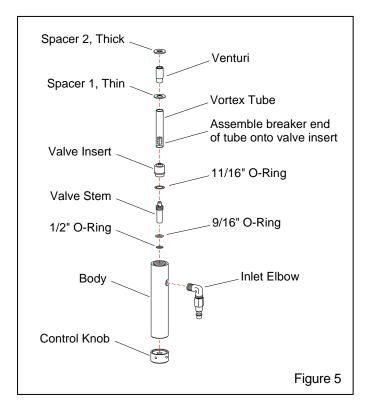
**5.3.2** Unscrew the valve stem from the valve insert and remove the two o-rings.
