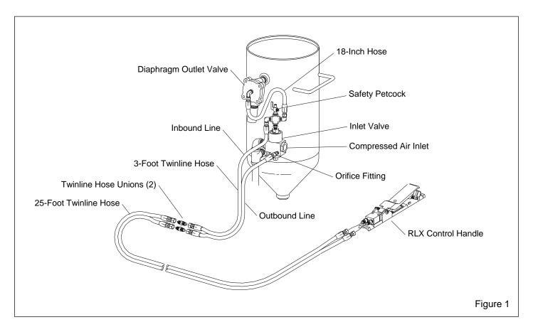
**1.3.4** TLR-50 Remote Controls are pressure-release style systems which control the pressurization and depressurization of the blast machine. Pressurization occurs when the control handle is pressed and depressurization occurs when the handle is released.
