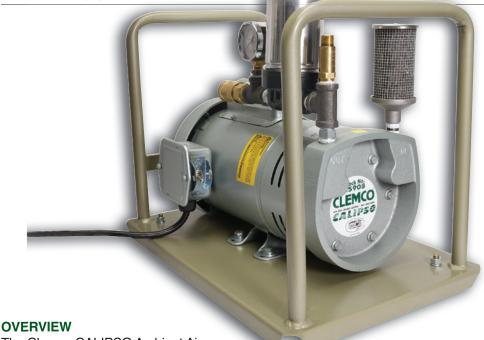
The Clemco CALIPSO Ambient Air Pump conveys breathing air from a clean environment outside the work area to a low-pressure type CE supplied-air respirator worn by an operator inside the work area without introducing oil or other contaminants.
