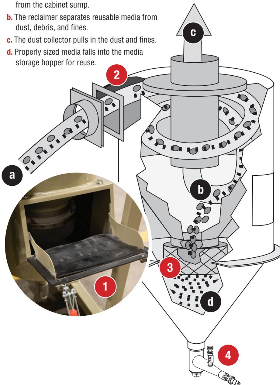
**The media reclaimer maintains an effective media working mix while simultaneously removing dust and debris from the blast system. This process ensures consistent blasting results and peak blast system performance.**
