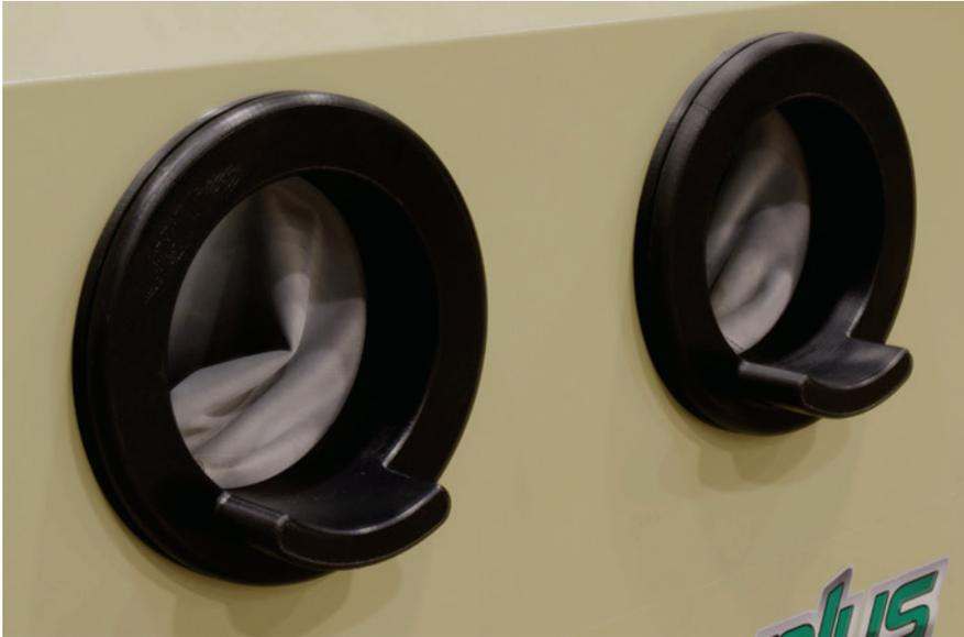
**Ergonomic glove ports and height-adjustable, electric lift legs are examples of Pulsar Plus innovations that helped create this efficient, durable, operator-friendly line of blast cabinets.**
