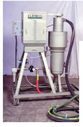
Super Comet with inside angle brush cleans a path 1-inch wide up to 72 inches per minute
