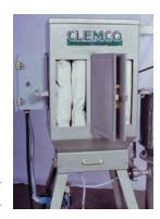
The Super Comet pressure-blast system delivers an enclosed high-velocity stream of abrasive to the surface being cleaned. The closed-circuit blast head features a 3/16-inch nozzle and multiple brushes for cleaning inside and outside angles, and uneven surfaces. It cleans a path about 1-inch wide up to 72 inches per minute, consuming 45 cfm when the nozzle is new and up to 70 cfm when worn, at 80 psi.
