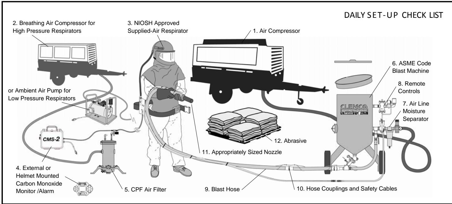
Make sure all blast operators are properly trained and suitably attired with a blast suit, safety boots, leather gloves, respiratory and hearing protection. Every day before start up, check all equipment components, including piping, fittings, and hoses, and valves, for leaks, tightness, and wear. Repair or replace as needed. Use the following checklist.
