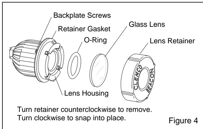
**5.1.2** If the retainer cannot be turned, loosen the four backplate screws several turns to remove compression from the retainer gasket, then remove retainer. NOTE: when the gasket is compressed as described in Paragraph 5.1.6, friction against the gasket may prevent the retainer from turning; loosening the backplate screws decompresses the gasket.
