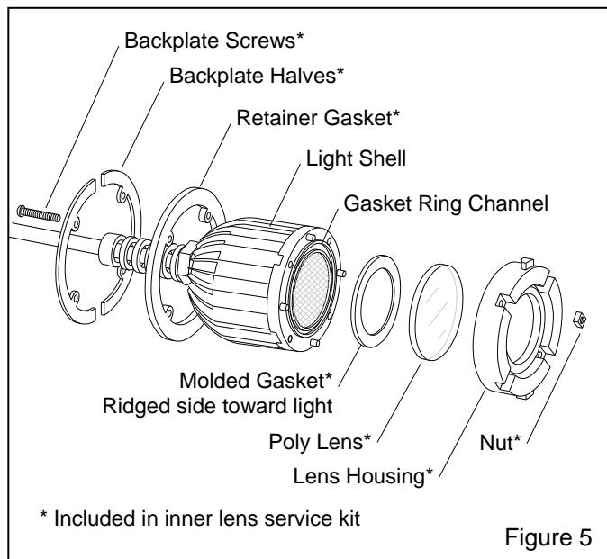
**5.2.3** Remove the lens housing from the light assembly. NOTE: The lens housing is held to the light shell by friction. Pull the housing to remove it from the shell; cup the housing when removing it to catch the inner lens, it is loose within the housing.
