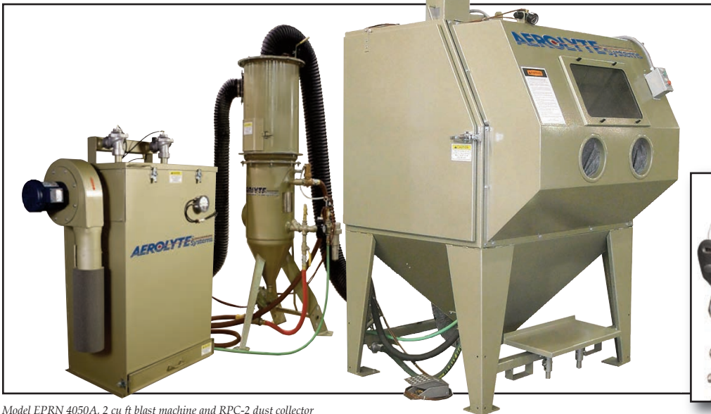
Model EPRN 4050A, 2 cu ft blast machine and RPC-2 dust collector
