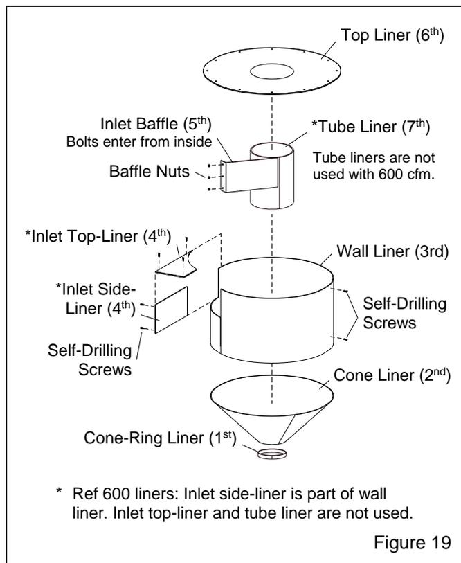
Installation Note: The numbers in parenthesis (-) shown in Figure 19 and the applicable paragraph, show the recommend order of installation. When installing liners, make sure that seams are aligned. The final assembly must be smooth and free of protrusions, edges, and gaps. Any edges will disrupt the air flow, causing wear, and affect the reclaimer's media cleaning efficiency.
