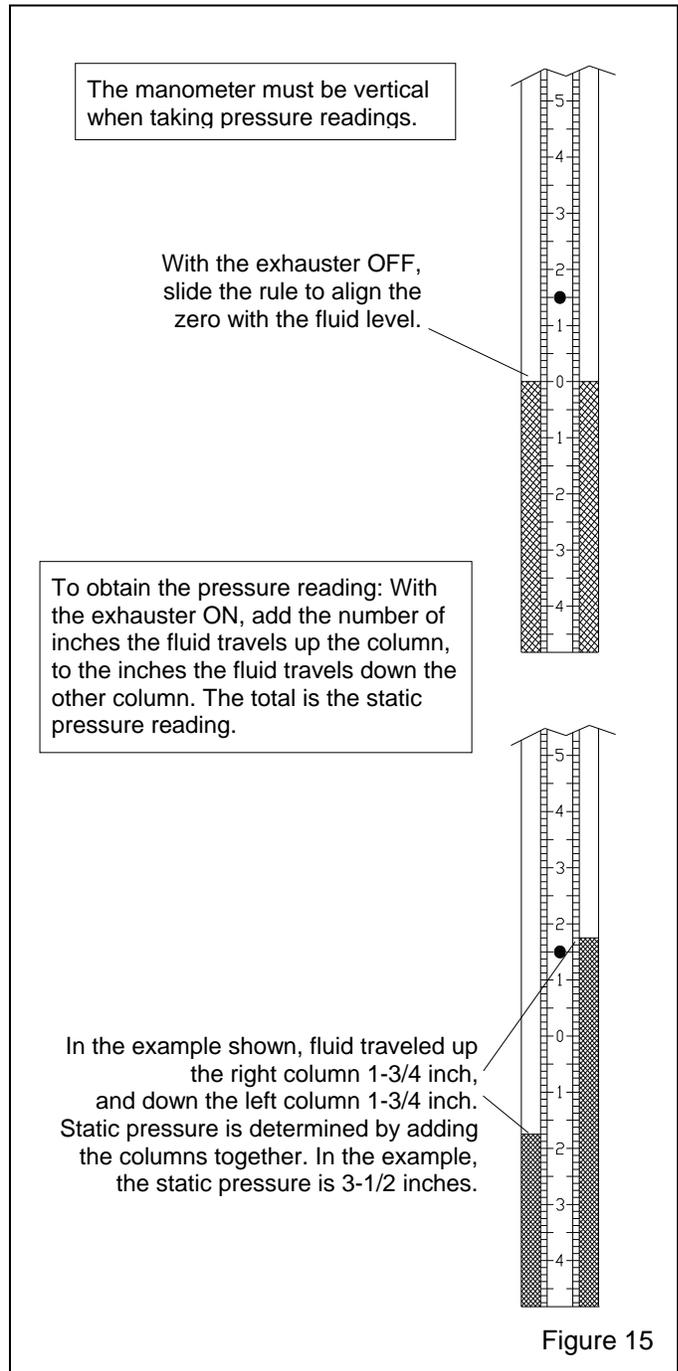
**5.10.7** Adjust the slide rule to align the zero with the fluid level. Refer to Figure 15.
