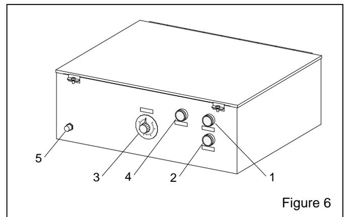
**3. Timer:** Sets duration of the blast cycle. Turn the dial to set the blast duration between 1 minute and 60 minutes. Once the timer is set, begin blasting by pushing the "System Start" button. Blasting automatically stops when the timer times-out. The time must be reset after every blast cycle.
