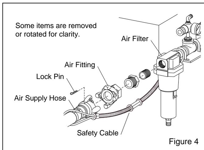
2.4.2 Connect an air line from the air source to the air filter inlet. For best blasting performance, size the air line as follows:
