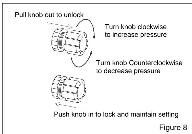
**5.1.2** To adjust, unlock the knob, and turn it clockwise to increase pressure or counterclockwise to decrease pressure. Pressure will usually drop from closed-line pressure when blasting starts. Once operating pressure is reached, lock the knob to maintain the setting
