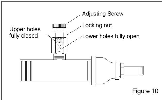
**5.3.3** If pulsation occurs in the media hose, either media is damp and caked, or not enough air is entering the media stream. While blasting, loosen the locking nut and slowly turn the adjusting screw out (counterclockwise when viewed from the top) until the media flows smoothly. Tighten the locking nut finger-tight to maintain the setting.
