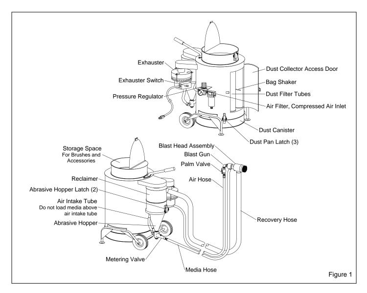
**1.4.6** Air, dust and fine by-products leave the reclaimer and are drawn through the dust collector. Dust collects in the cloth filter, and the cleaned air passes through the exhaust fan and is discharged into the atmosphere. Dust particles trapped by the filter bags are removed by a mechanical bag shaking mechanism; dust released from the bags collects in a removable canister for disposal.
