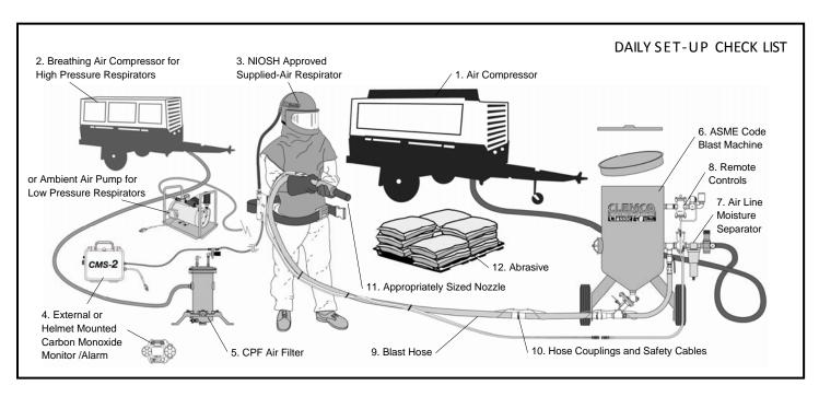
Make sure all blast operators are properly trained and suitably attired with a blast suit, safety boots, leather gloves, respiratory and hearing protection. Every day before start up, check all equipment components, including piping, fittings, and hoses, and valves, for leaks, tightness, and wear. Repair or replace as needed. Use the following checklist.
