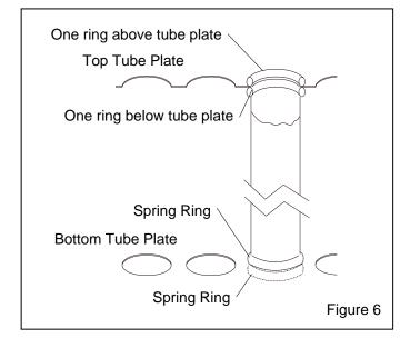
**6.2.2** The tubular filters are held firmly by a spring ring above and below the perimeter of the hole in the plate. The other end of the filter is similarly installed in the lower plate. The filters must fit tightly to prevent dust leakage. To ensure a tight seal, apply force as necessary. Check for proper seating at both ends, and remove any twist before proceeding to the next filter.
