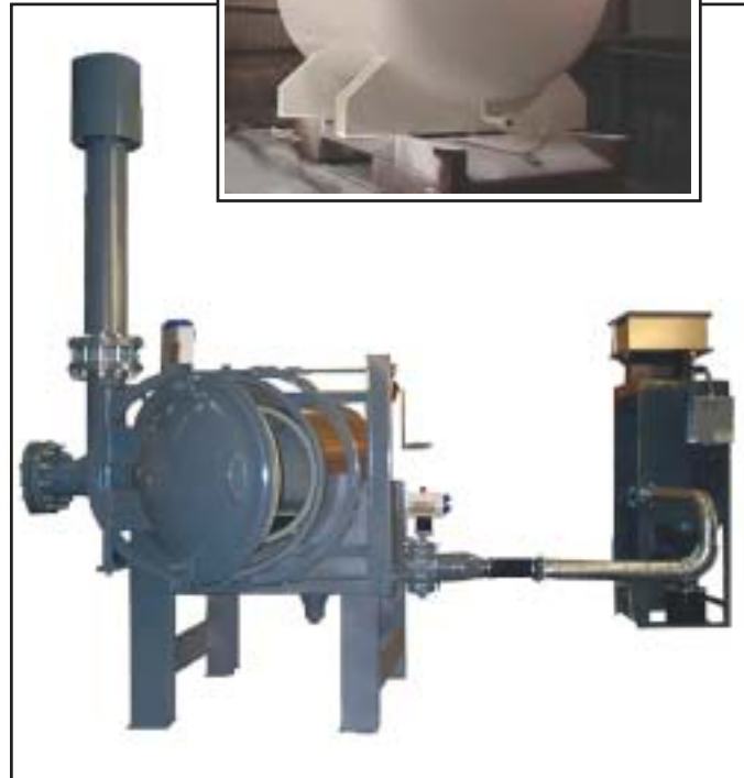
1/4-Pound Shape-Charge Test Chamber with Emission Treatment to Meet California EPA Requirements
