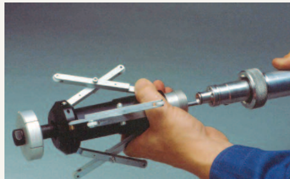
Orbiter I coats 3.5-inch through 7-inch pipes.
